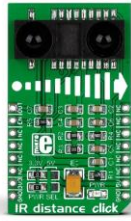
Fig. 2. IR distance click - distance measuring sensor, which comprises of an integrated PSD (position sensitive detector), an infrared LED and a signal processing circuit.
