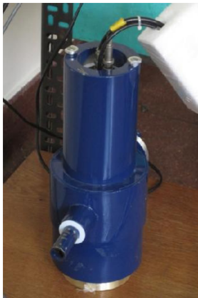
Fig. 2. Experimental setup: detector and sample holder in the lead collimator
