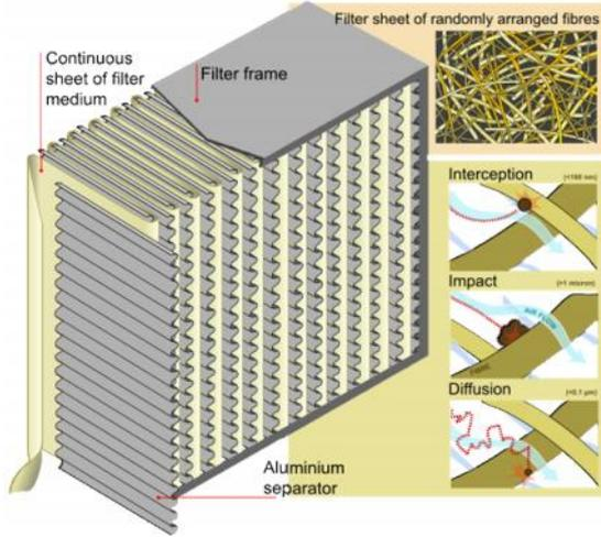
Fig. 5. Schematic view of measured HEPA filter
