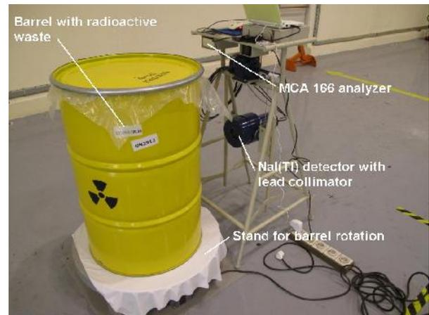
Fig. 4. Standard metal barrel with radioactive waste
