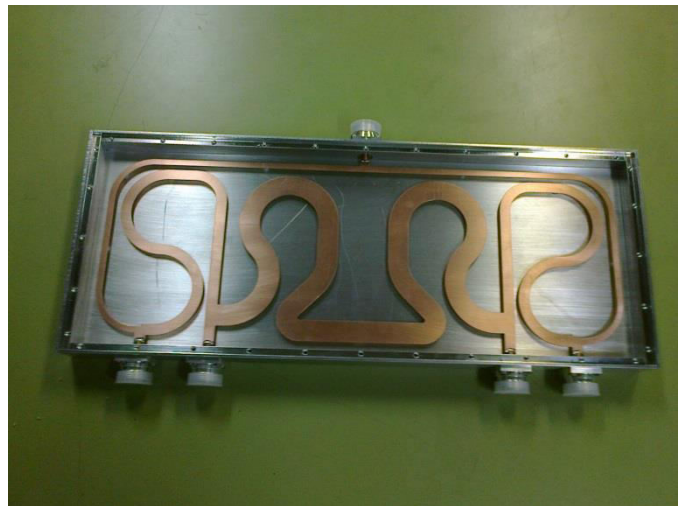
Fig. 4. The picture of the produced Gysel 3dB power divider/combiner.
