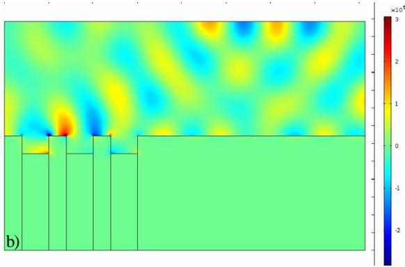
Fig. 4. Electric field spatial distribution for  $d_1 = 200$  nm,  $d_2 = 300$  nm and  $d_p = 4\lambda$  structure at 642 nm and  $30^\circ$  incident angle; a) electric field intensity, b) component of the electric field vector in direction perpendicular to the surface.
