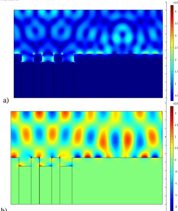
Fig. 5. Electric field spatial distribution for  $d_1 = 200$  nm,  $d_2 = 300$  nm and  $d_p = 4\lambda$  structure at 552 nm and normal incidence; a) electric field intensity, b) component of the electric field vector in direction perpendicular to the surface.
