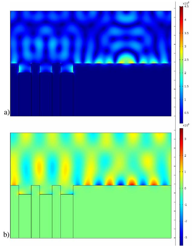
Fig. 3 Electric field spatial distribution for  $d_1 = 200$  nm,  $d_2 = 300$  nm and  $d_p = 4\lambda$  structure at 584 nm and normal incidence; a) electric field intensity, b) component of the electric field vector in the direction perpendicular to the surface.
