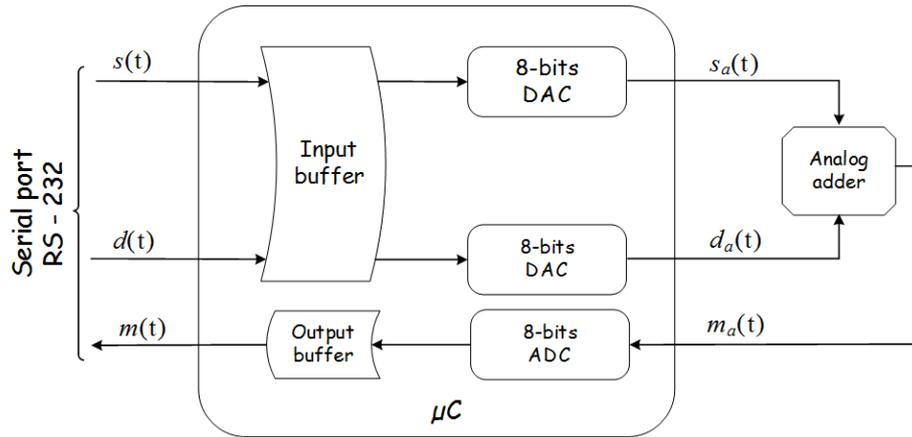
Fig. 3. The functional block-scheme of the experimental PCB which is connected with PC through the serial port RS-232, where  $s(t)$  is input signal,  $d(t)$  is dither and  $m(t)$  is the resulting signal.
