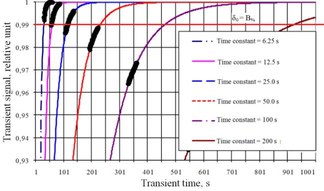
Fig. 3. Observation interval position on the transient curves with different time constants.
