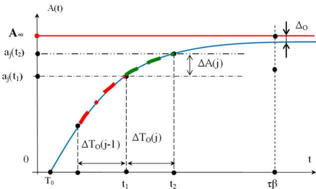
Fig. 1. Position of the observation interval on the transient curve.
