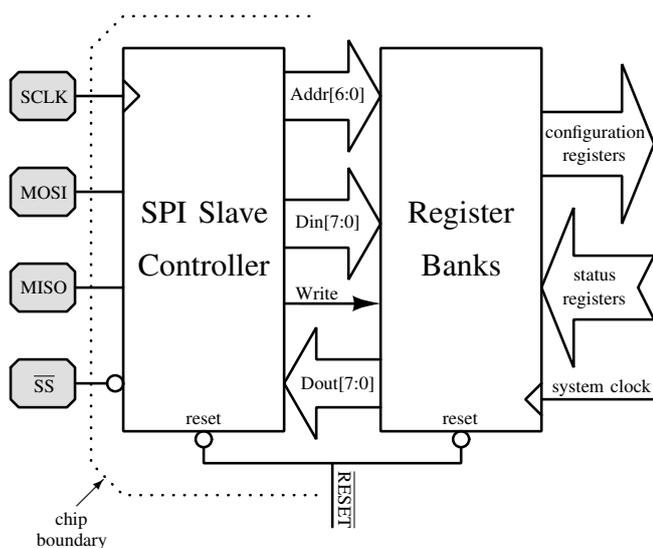
Fig. 7. A simplified SPI slave controller and its register bank interconnection.
