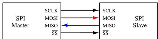
Fig. 1. A basic SPI bus example of Single SPI Master to Single SPI Slave.
