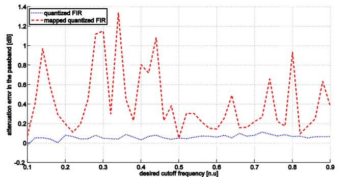
Fig. 6. Mean value of degradation of passband attenuation in low pass filters due to quantization, in the case of direct form realization (blue dotted), and transformed realization (red dashed).
