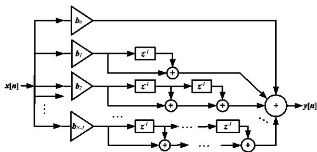
Fig. 1. Filter realization structure based on polynomial basis transform [6].
