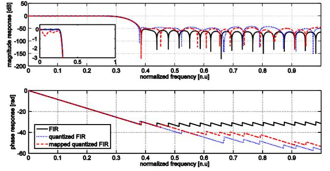
Fig. 4. Magnitude and phase responses of a low pass filter with  $\omega_{des}=0.32\pi$ , showing desired characteristics (black solid), direct form realization with quantized coefficients (blue dotted), and transformed realization with quantized coefficients (red dashed).
