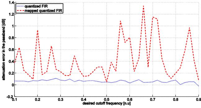
Fig. 7. Mean value of degradation of passband attenuation in high pass filters due to quantization, in the case of direct form realization (black solid), and transformed realization (blue dotted), and mapped realization (red dashed).
