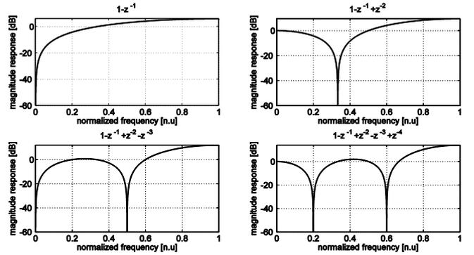
Fig. 3. Magnitude responses of base polynomial filters for high pass filter design.
