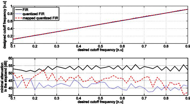
Fig. 9. Designed cutoff frequencies (upper subplot) and minimal attenuations in the stopband (lower subplot) of high pass filters, in the case of desired filter (black solid), direct form realization with quantized coefficients (blue dotted), and transformed realization with quantized coefficients (red dashed).
