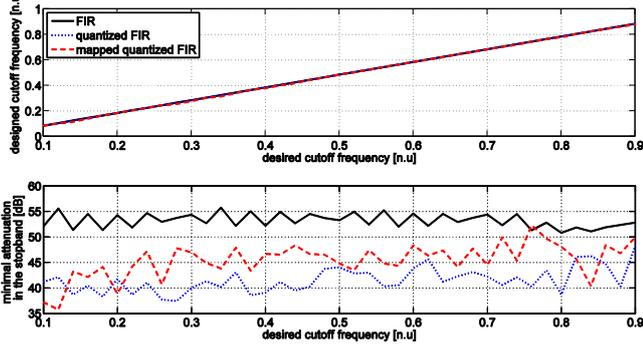
Fig. 8. Designed cutoff frequencies (upper subplot) and minimal attenuations in the stopband (lower subplot) of low pass filters, in the case of desired filter (black solid), direct form realization with quantized coefficients (blue dotted), and transformed realization with quantized coefficients (red dashed).
