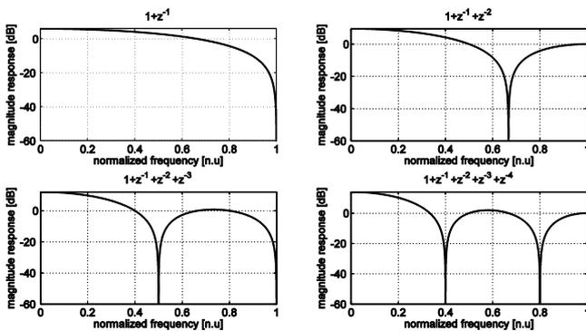
Fig. 2. Magnitude responses of base polynomial filters for low pass filter design.
