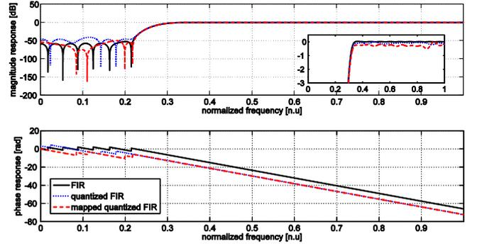
Fig. 5. Magnitude and phase responses of a high pass filter with  $\omega_{des}=0.28\pi$ , showing desired characteristics (black solid), direct form realization with quantized coefficients (blue dotted), and transformed realization with quantized coefficients (red dashed).
