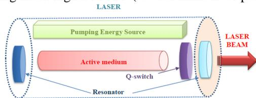
Fig.2. Solid State Laser Structure
