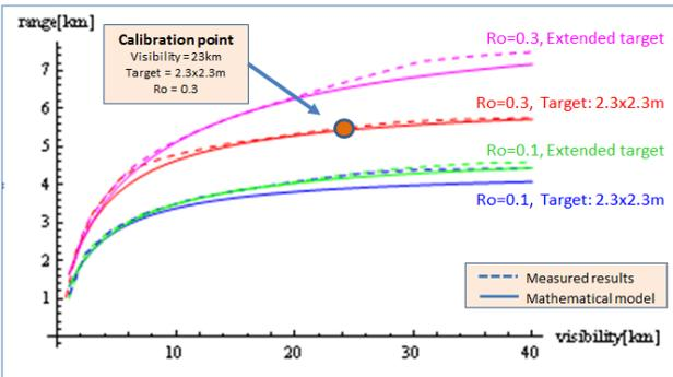
Fig.5. LRF range versus target size and meteorological visibility
