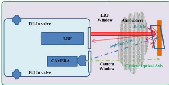
Fig.7. Field based System bore sighting definition and principles
