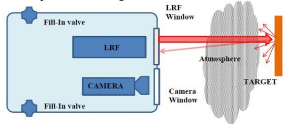
Fig.6: Distance Measurement sub-system structure
