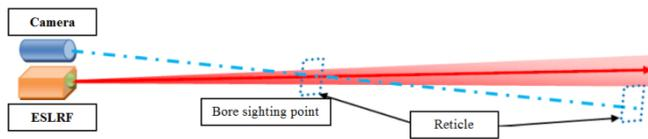
Fig.8. Reticle position during bore sighting and distance measurements
