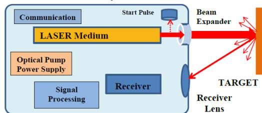
Fig.3. LRF based Distance Measurement Process
