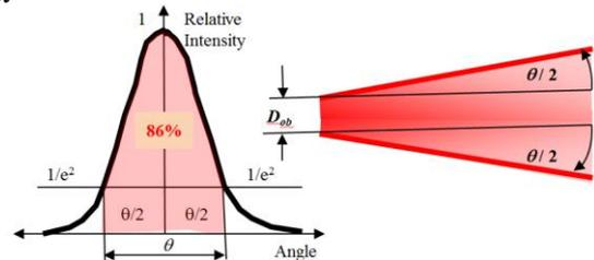
Fig.4. Gaussian laser beam parameters (diameter and divergence)
