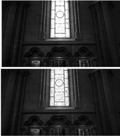
Figure 1. Low dynamic (upper) and high dynamic range grayscale image tone mapped by the Reinhard approach (lower).
