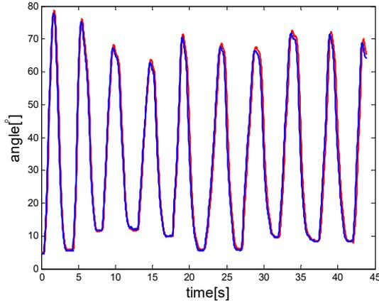
Fig. 6. Angle detected from camera and joint angle encoder for ten repetitions of a full knee extension. A red line shows the camera detected angle and the blue line are signals from the joint angle encoder.
