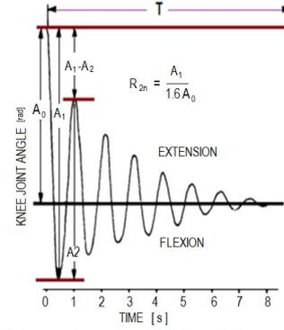
Fig. 2: The sketch of the goniogram of the knee joint and the parameters that are quantifying spasticity [3, 5]
