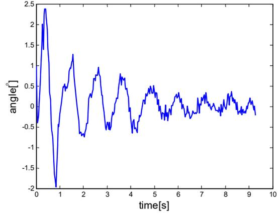
Fig. 9. An example of the error during the pendulum test: the difference between the goniograms from the image analysis and the joint encoder.
