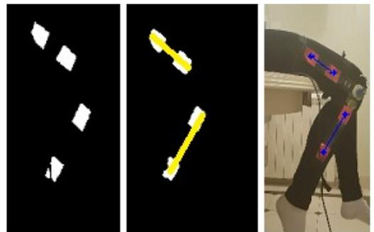
Fig. 5. The reconstructed image after the threshold=30 was applied and the same image after morphological operations (left panels). The image shown in Fig. 3 with the centroids detected and the lines defining the directions of the thigh and the shank
