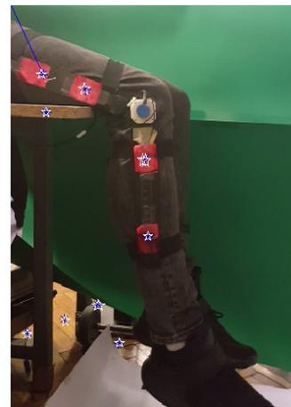
Fig. 10: False detected markers due to inadequate background marked with asterisks.
