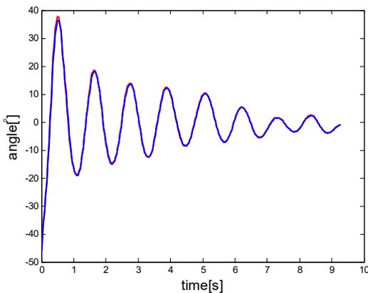
Fig. 8. An example of the knee joint goniogram estimated by image analysis of the movie recorded (red) and the signals from the joint angle encoder (blue) for the pendulum test.
