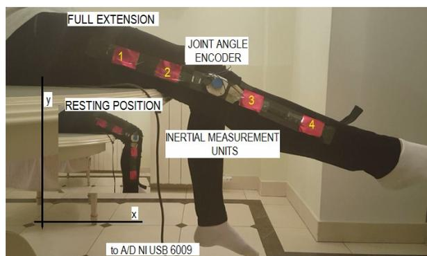
Fig. 1. The neutral position of the leg (insert) and the fully extended leg. Four red markers are used for the image based estimation of the movement. Hall-effect based absolute angle encoder and spatial inertial measurement units (accelerometers and gyroscopes) are components of the pendulum test apparatus described in Popović-Maneski et al. [5].
