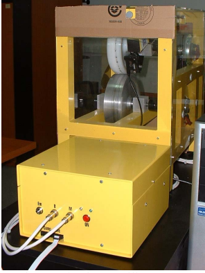
Fig. 5. ABS experimental setup in the Intelligent Control Systems Laboratory of the Politehnica University of Timisoara, Romania [67].
