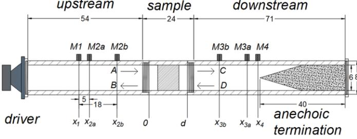
Fig. 2. Cross-section of the device. Microphone positions, construction elements and most important dimensions are shown.
