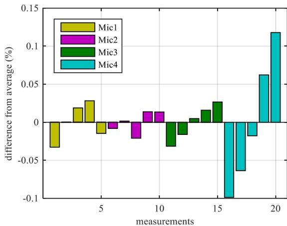
Fig. 8. Repeatability of magnitude of IRs (measured by all 4 microphones placed in the position of the microphone 1 and repeated 5 times) calculated as a difference from the average magnitude value.
