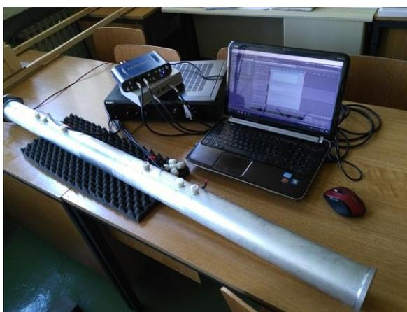
Fig. 6 Measurement setup for recording inside the tube.
