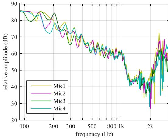
Fig. 11. Frequency response recorded at 4 microphone positions in the case of empty tube
