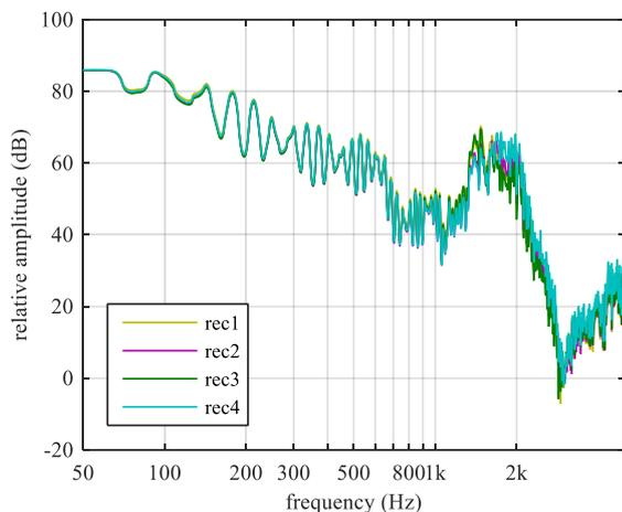
Fig. 9. Repeatability of IRs frequency response of 4 microphone, measured in position M1.
