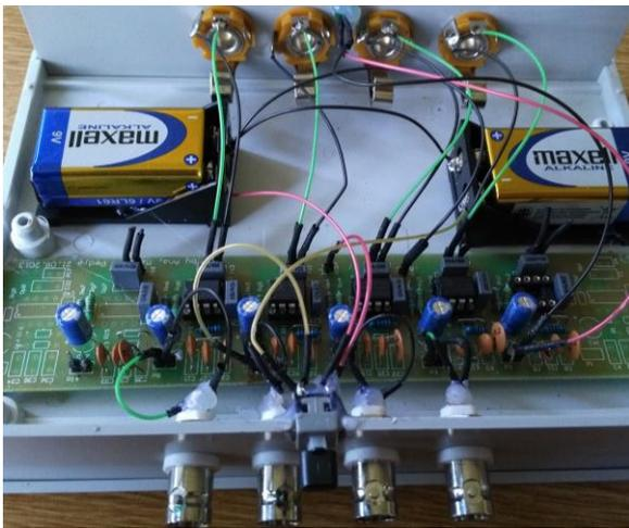
Fig. 3. Inside look of the preamplifier circuit box. Connectors, wiring, SSM2019 and battery power can be seen. Four channels are connected.
