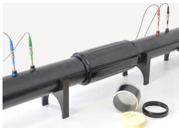
Fig. 1. Commercially available transmission loss tube by “Akustik Dorschung Dresden”
