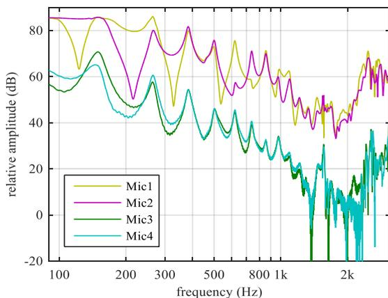
Fig. 13. Frequency responses of signals (IRs) recorded at 4 microphone positions in the case of sample placed in a middle section of the tube
