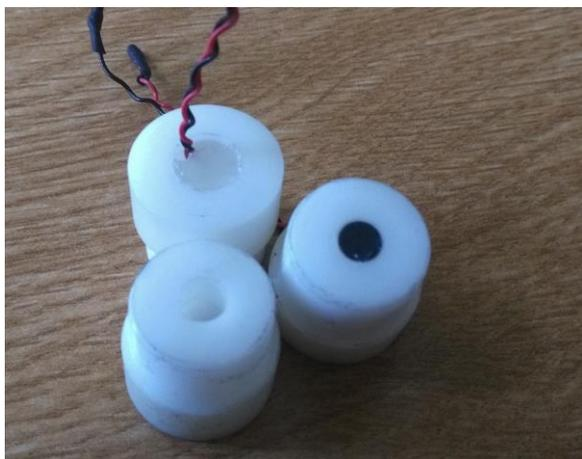
Fig. 5. Microphone elements fitted to the casing. Wires movement is restricted with silicon glue.
