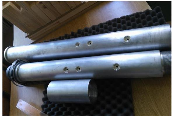
Fig. 4. Components of the tube, *upstream*, *downstream* and middle section tubes.
