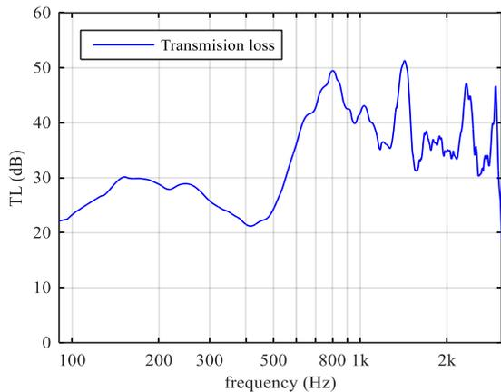
Fig. 12. TL calculated using microphone pairs  $M1-M2b$  and  $M4-M3b$
