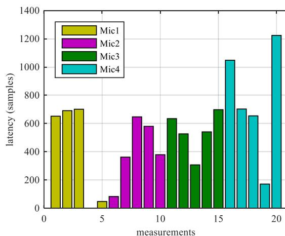
Fig. 7. Repeatability of IRs (measured by all 4 microphones placed in the position of the microphone 1 and repeated 5 times) regarding relative latency presented as a difference from the least delayed IR. Sampling frequency of 44.1 kHz was used.
