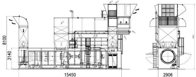
Fig. 4. Generic configuration of a Solar Titan 130 Gas Turbine Generator package specified for an offshore facility.
