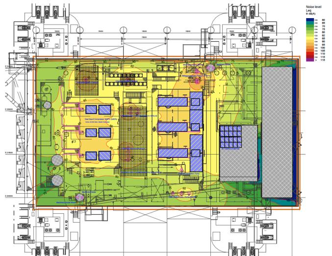
Fig. 7. Combined noise levels predicted on the Main Deck of an offshore platform. The noise sources comprise gas turbine generators, gas export compressors, pump packages (including motors) and piping.
