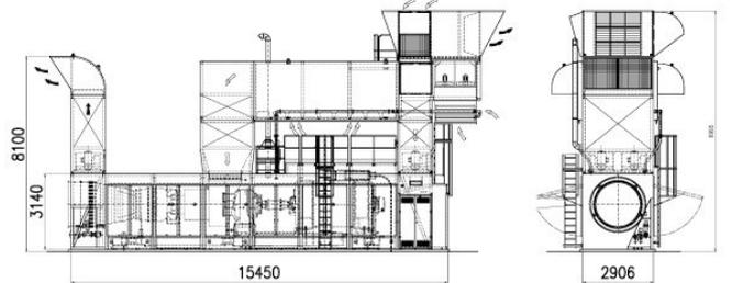
Fig. 4. Generic configuration of a Solar Titan 130 Gas Turbine Generator package specified for an offshore facility.
