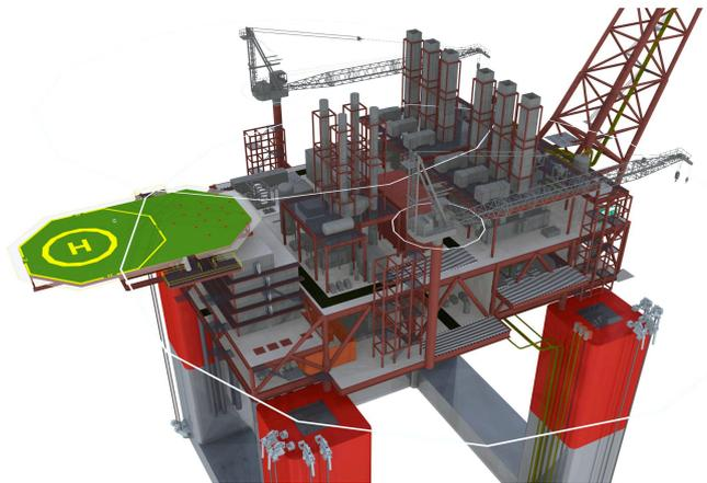
Fig. 1. A conceptual General Arrangement 3D model of an offshore facility depicting noisy equipment distributed across the sound-reflecting (plated) and sound-transparent (grated) platform decking.
