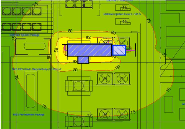
Fig. 8. Noise levels predicted on the Main Deck for an isolated GTG package comprising a number of point, line and area sources. Noise levels are over-predicted with the Traditional Method for ground effect attenuation.
