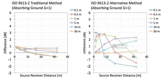
Fig. 6. Traditional vs. Alternative ground effect for soft (absorbing) ground: difference in dB between the theoretical free-field spreading and simulated total attenuation at various source-receiver heights and distances.
