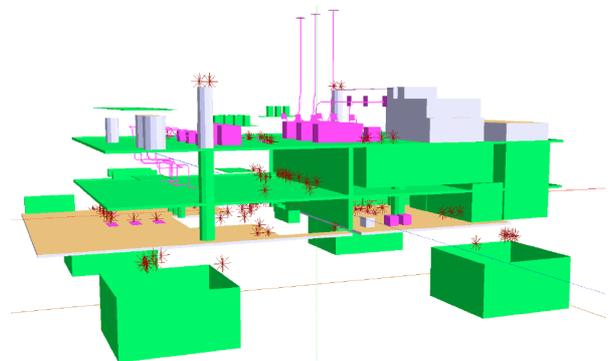
Fig. 2. An acoustical model of an offshore facility depicting elevated noise sources. For calculation purposes, the model was split into the Main Deck Model, Production and Mezzanine Deck Model and Hull Model.
