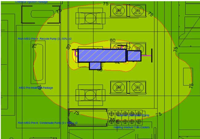
Fig. 9. Noise levels predicted on the Main Deck for an isolated GTG package comprising a number of point, line and area sources. Noise levels are realistically predicted with the Alternative Method for ground effect attenuation.
