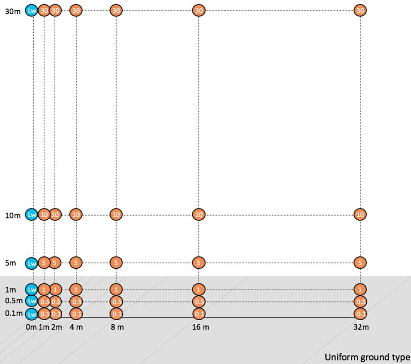
Fig. 3. Test Case source-receiver grid above a flat terrain with a uniform ground type (absorbing or reflecting).
