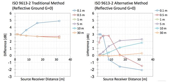
Fig. 5. Traditional vs. Alternative ground effect for hard (reflective) ground: difference in dB between the theoretical free-field spreading and simulated total attenuation at various source-receiver heights and distances.
