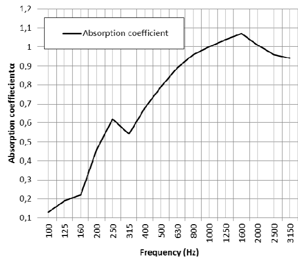
Fig. 7. Measured sound absorption coefficient \alpha of panel Tiho according to standard ISO 354.
