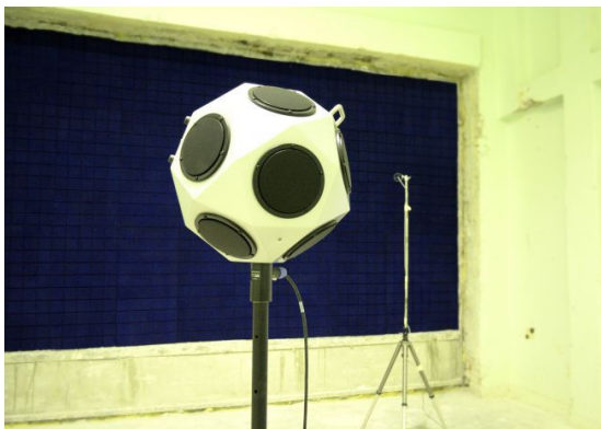
Fig. 5. Measurement of TL in laboratory with installed panels on the wall at the side of the receiver room.
