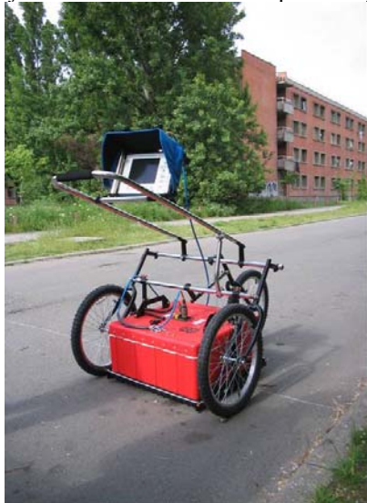
Sl. 11. Ground Penetrating Radar
