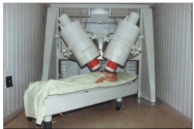
Fig. 3. The 2x31 channel biomagnetometer system in the magnetically shielded room at Biomagnetic Center Jena
