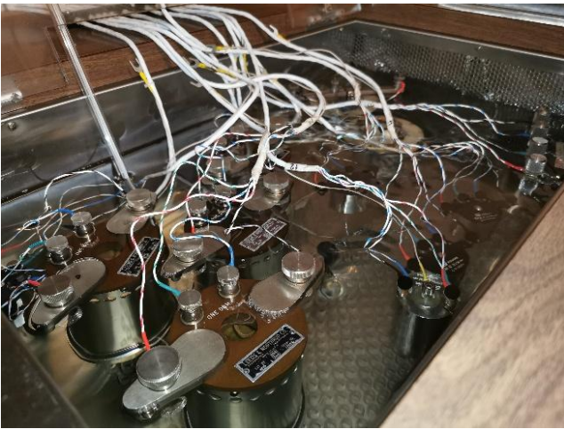
Fig. 1. Temperature stabilization of the standard resistors in an oil bath.
