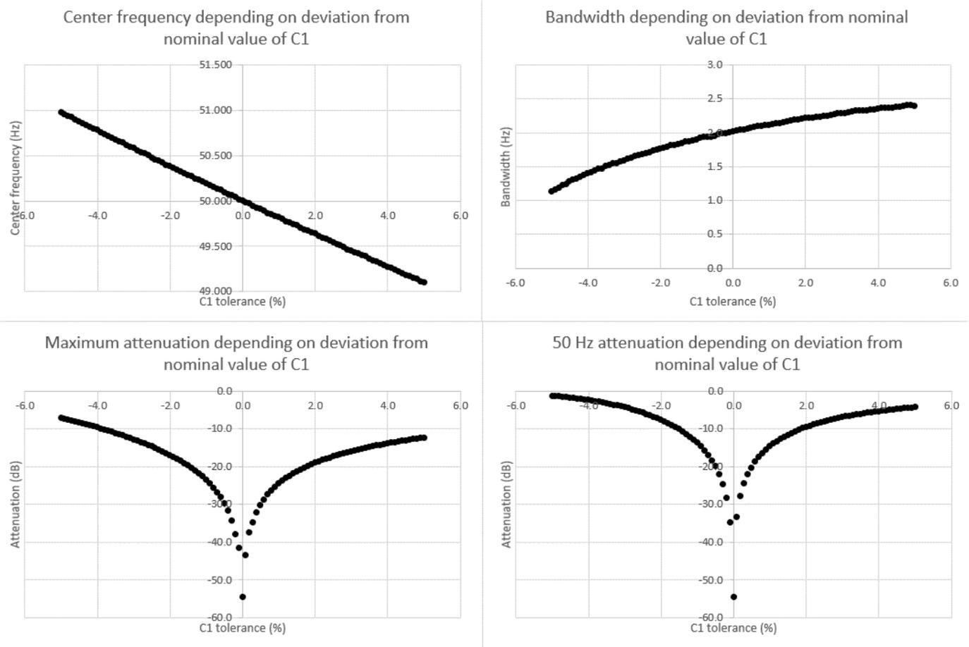
Fig. 5. Graphs showing impact of  $C_1$  tolerance on transfer function
