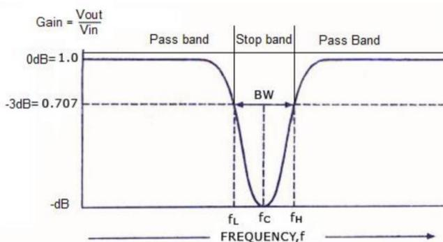
Fig. 1. General amplitude response of a band-stop filter [1]
