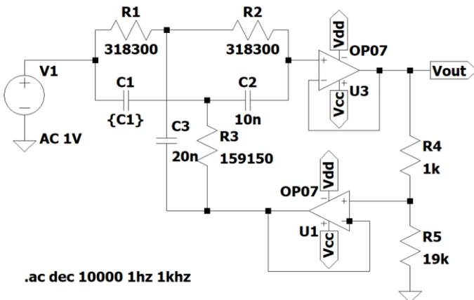
Fig. 3. 50 Hz notch filter in LTspice
