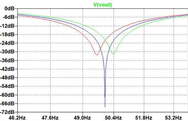
Fig. 4. Changes in twin T notch transfer function in respect to deviation of  $C_1$
