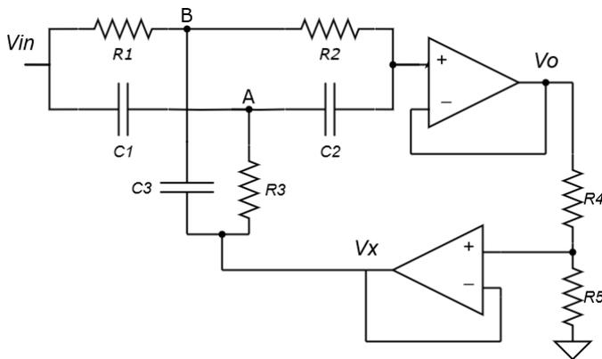
Fig 2. Active twin-T notch filter circuit
