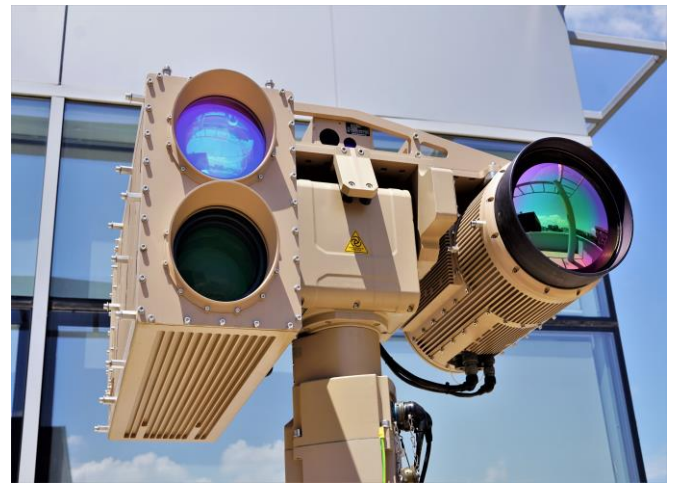
Fig. 2. Multi Sensor Imaging System on pan-tilt positioner, equipped with color, SWIR and thermal camera.
