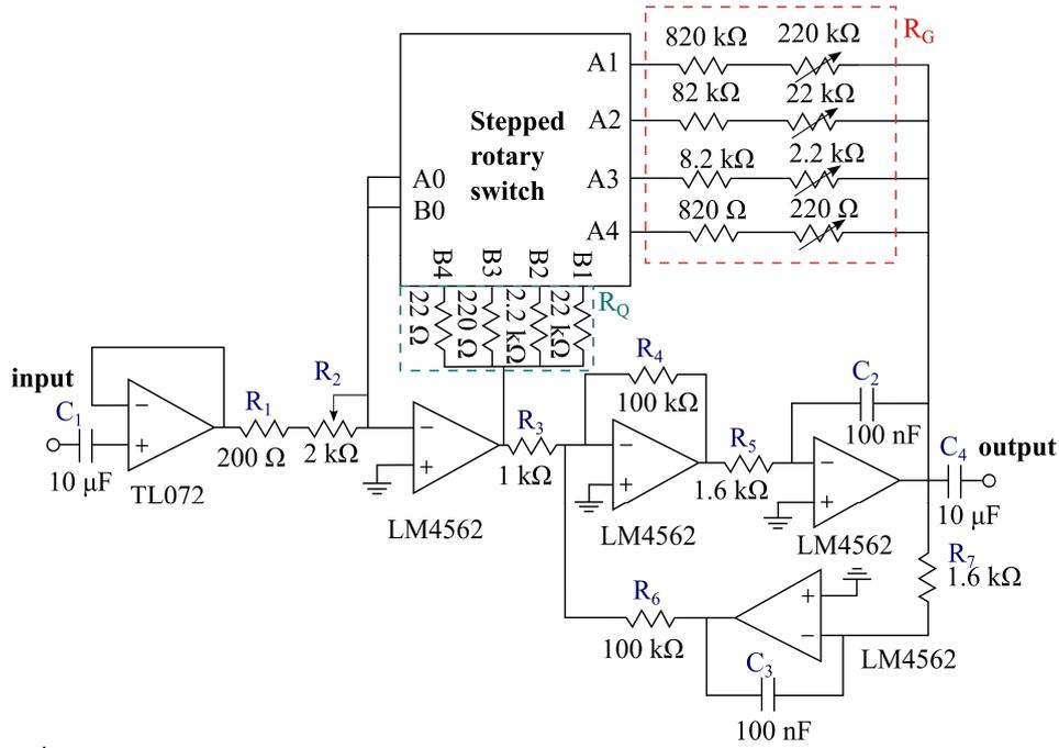
Fig. 1. SWR meter schematics.
