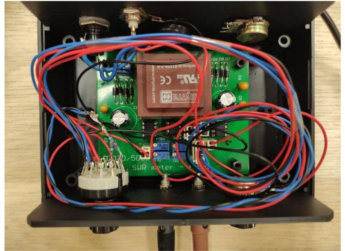
Fig. 3. The prototype of the SWR meter.
