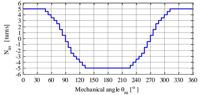
Fig.2. Stator phase A - winding function
