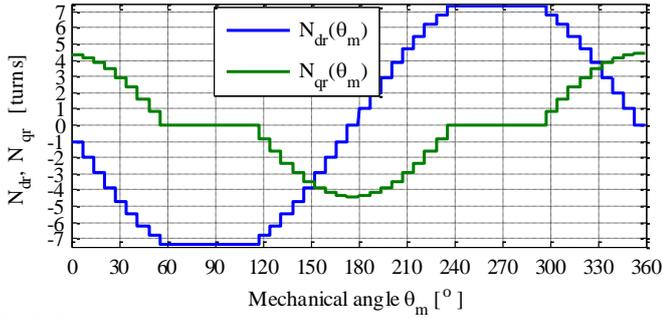
Fig.7. Damper winding functions along the  $d$  and  $q$  axes
