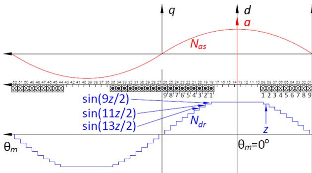
Fig.5. Damper winding function along the  $d$  axes
