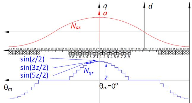
Fig.6. Damper winding function along the  $q$  axes
