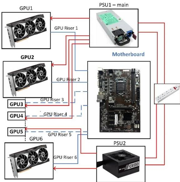
Fig. 7. Block scheme of the cryptocurrency mining rig
