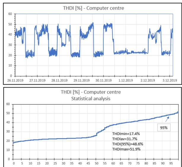
Fig. 6. Variation of the computer centre THDI during one-week measurements: time wave-form (up) and statistical analysis (down)
