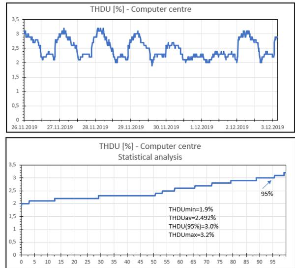
Fig. 5. Variation of the computer centre THDU during one-week measurements: time wave-form (up) and statistical analysis (down)
