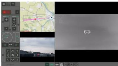
Fig. 3. Graphical user interface (GUI) of an operator's console, with two video streams, map, statuses and controls.
