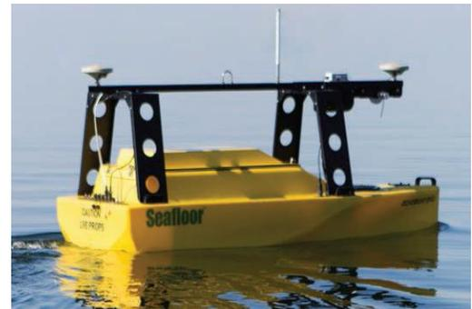
Fig. 8. EchoBoat-240 seafloor system [13]
