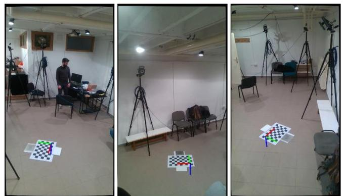
Fig 2. Images used for extrinsic camera calibration displayed with system origin
