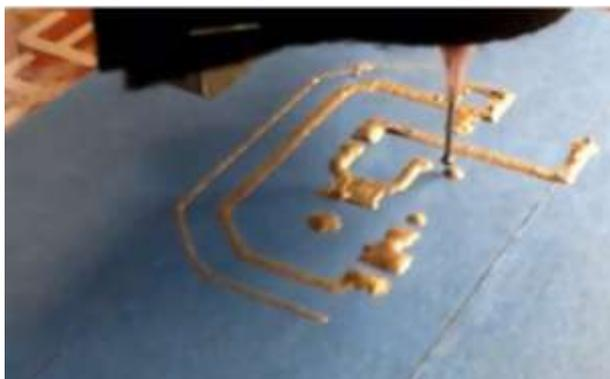
Fig. 3. Results after applying the 3D printing method with using the golden wire in production of one circuit board: a) correct and b) incorrect
