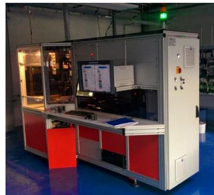
Fig. 13 Robotized system for current transformers accuracy testing in MBS factory Germany (2012.) [54]
