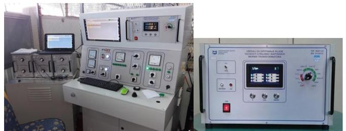
Fig. 14 Automatic device for accuracy testing of 3 current transformers simultaneously [55]
