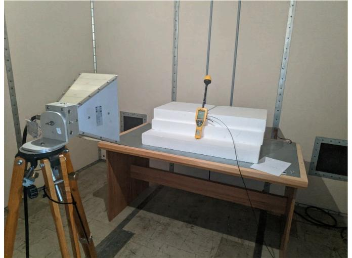
Fig. 3. Electric field strength measurement with electric field meter, double-ridge transmitting antenna.
