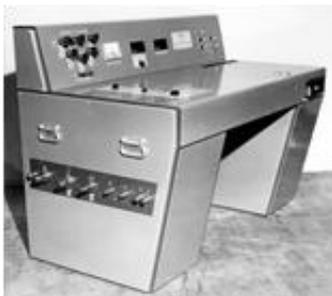
Fig. 11 System for automatic accuracy testing of current measuring transformer, type ASK-1 [52]
