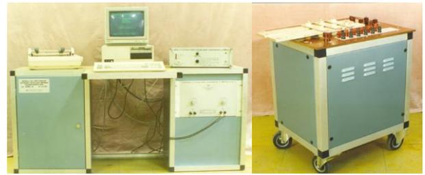
Fig. 12 System for automatic accuracy testing of current measuring transformer, type ASK-2 [53]
