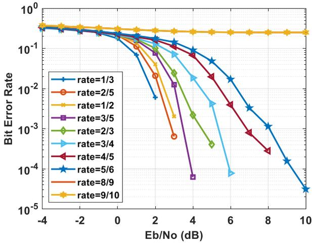
Fig. 2. LDPC - BER performance for variable code rates
