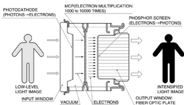
Fig. 1. Image intensifier tube operating principle [3].
