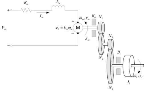
Fig. 1. SRV02 DC motor armature circuit and gain train [11]
