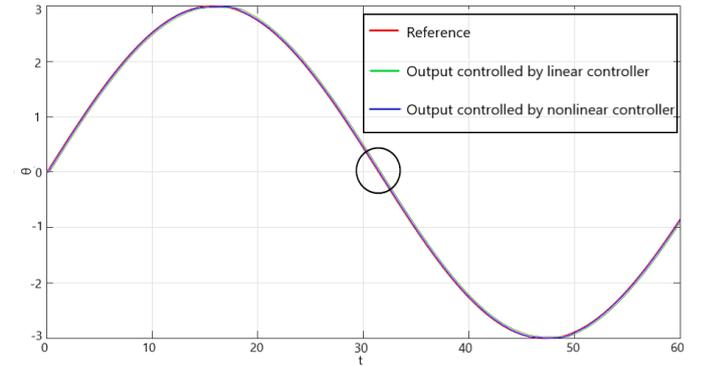
Fig. 10. Experimental results: position tracking of sine signal for the linear and nonlinear controller
