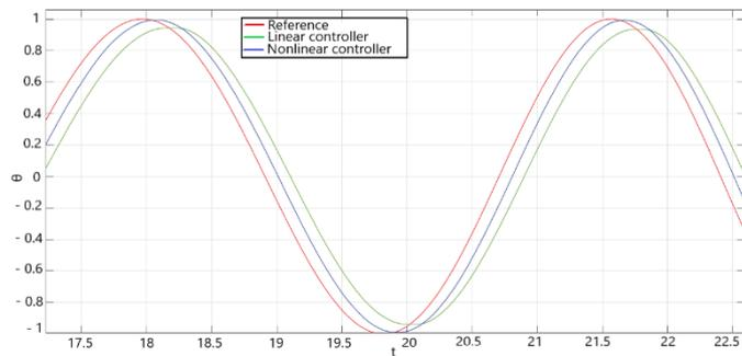
Fig. 12. Experimental results: position tracking of chirp signal for the linear and nonlinear controller
