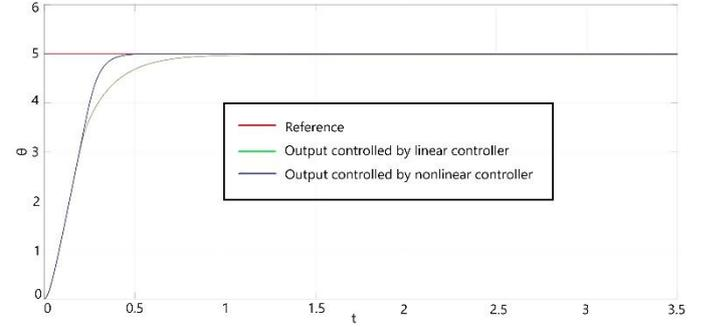
Fig. 9. Experimental results: position tracking of step signal for the linear and nonlinear controller
