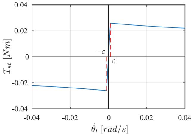
Fig. 5. Friction characteristics of DC motor [14]
