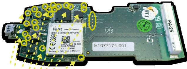
Test points on the boards that went through the whole testing and production process
